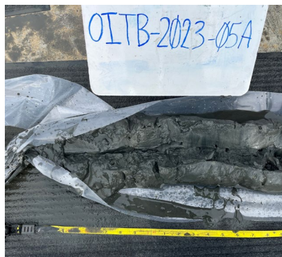
OITB-2023-05A (0 TO 2.1 FEET) Top of core to approximately 2.1 feet below mudline. Collected via vibracore.
