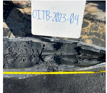
OITB-2023-04 (6.8 TO 9.4 FEET) Photo depth to approximately 9.4 feet below mudline (approximate bottom of core). Collected via vibracore.
