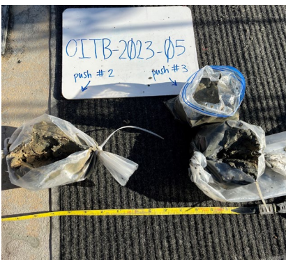
OITB-2023-05 (0 TO 0.5 FEET) Photo depth to approximately 0.5 feet below mudline for attempt #2 (left) and attempt #3 (right). Collected via vibracore.
