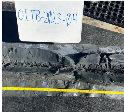
OITB-2023-04 (4.4 TO 6.8 FEET) Photo depth to approximately 6.7 feet below mudline. Collected via vibracore.
