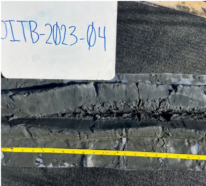
OITB-2023-04 (2.9 TO 5.1 FEET) Top of core to approximately 5.1 feet below mudline. Collected via vibracore.
