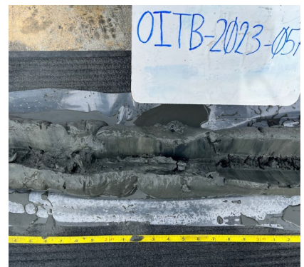
OITB-2023-05A (1.2 TO 3.4 FEET) Photo depth to approximately 3.4 feet below mudline. Collected via vibracore.
