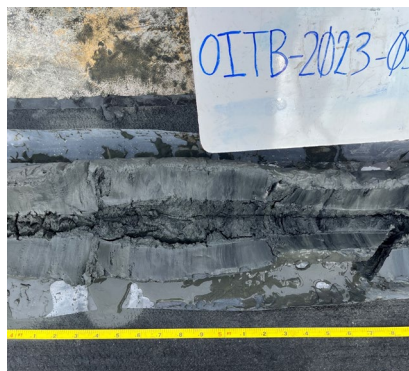
OITB-2023-05A (3.8 TO 6.1 FEET) Photo depth to approximately 6.1 feet below mudline. Collected via vibracore.
