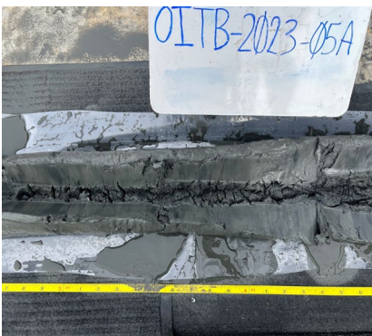
OITB-2023-05A (2.5 TO 4.7 FEET) Photo depth to approximately 4.7 feet below mudline. Collected via vibracore.
