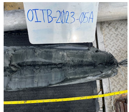
OITB-2023-05A (5.8 TO 8 FEET) Photo depth to approximately 8 feet below mudline (approximate bottom of core). Collected via vibracore.
